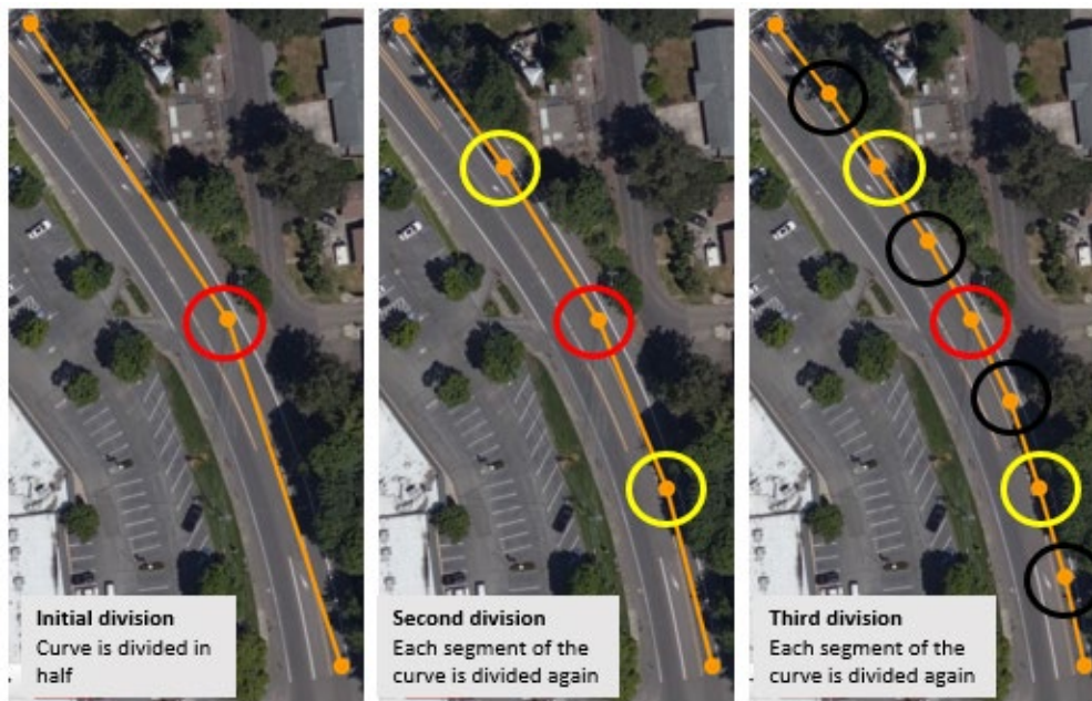
Figure 13: Node spacing in horizontal curves
