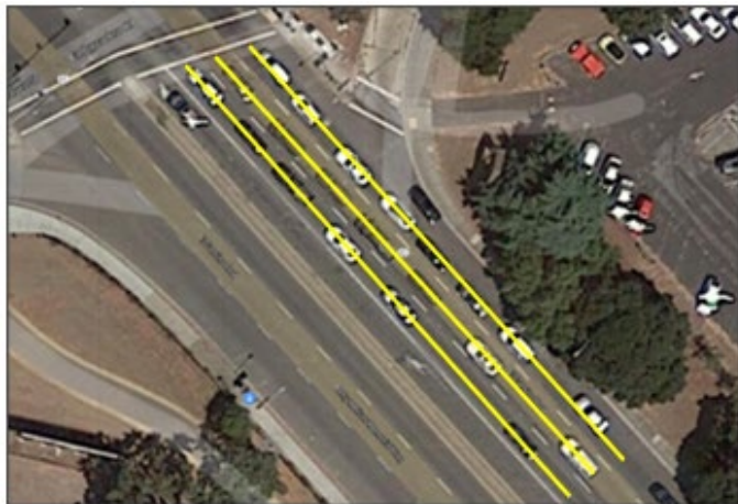
Figure 5: Yellow line overlayed on three straight parallel ingress lanes that match criteria for computed lanes Map source: Google Maps, Drawing source: Athey Creek Consultants
